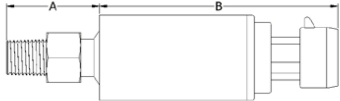
P10 - with Packard Metripack 150 (mates with Packard 12065287)
